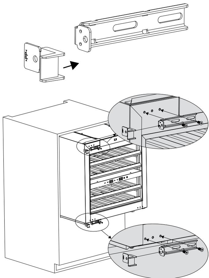
8. Slide the appliance until it is completely in the cabinet. Check all the gaps around the appliance. Use the spacers to position the appliance flush to the front of the cabinet. Loosen the screws (1), slide the spacers towards the side of the cabinet and then continue tightening the screws.
