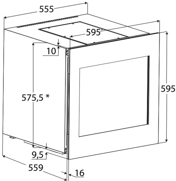
\*The adjustable feet can be used to increase the installation height to max. 590.5 mm.
