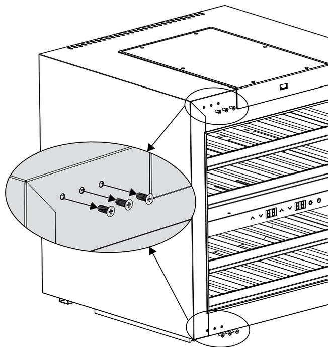
7. Place the spacers on the mounting brackets and screw them together. The position will vary depending on which way the door opens.
