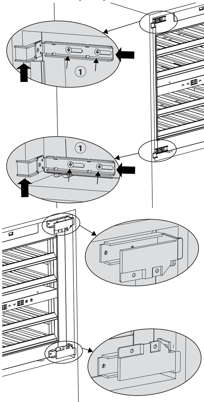
9. Secure the appliance to the kitchen cabinet by pushing the supplied screws through the spacers and the mounting brackets.
